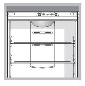
The No Frost system circulates cold air continuously to collect humidity and prevent ice and frost formation. The system maintains an optimal humidity level in the compartment, preserving the original quality of the food, preventing the food from sticking together and
