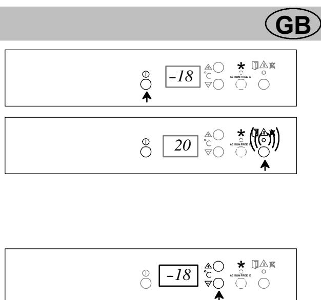
Once set, the temperature display shows the current temperature inside the freezer. Allow the cabinet to run for a period of 24 hours whenever the temperature setting is changed. This will allow the temperature to stabilise inside the cabinet. It is not necessary to reset the temperature when the cabinet is switched on after it has been out of use. The electronics recalls the previously set temperature.
