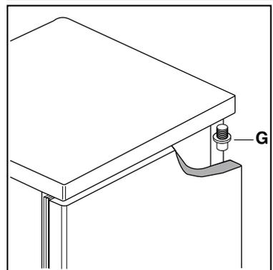
12. Unscrew the top handle bracket from the handle rod (1). Unscrew the bottom handle bracket from the door (2).
