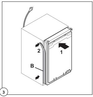
**N.B.** The joint cover (B) is to be assembled after having installed the appliance in the recess.
