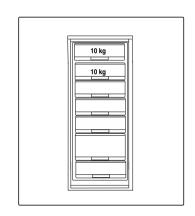
In order to freeze the quantity indicated on the rating plate, arrange the food directly in contact with the cooling surfaces. If the food is frozen in the baskets, the maximum quantity freezable is slightly less.
