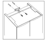
• The top of the appliance must be kept clear to allow correct air circulation. If a wall unit is fitted above the appliance, there must be a gap of 50 mm between this unit and the wall and it must be at least 50 mm below the ceiling.
