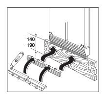
• If using a 100 mm plinth, fit the complete height compensation strip.
