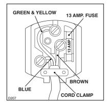
Connect the Green and Yellow (earth) wire to the terminal in the plug which is marked with the letter
