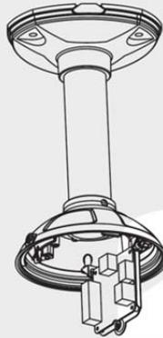
③ Hook up "Drop Prevention Spring" on main body to prevent camera from unexpected drop and connect Main Body Cable to Main Body Connector in Ceiling Mount Bracket.
