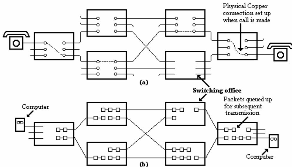
a) Circuit Switching b) Packet Switching
