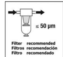
The air pressure supply must be clean (Filter < 50 µm)
