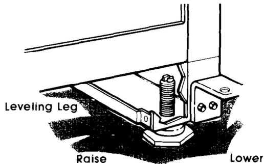
This freezer has 2 threaded leveling legs that are shipped in a separate package.
