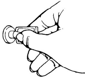
To lock or unlock the freezer you must hold the key in the lock while turning. The lock is spring loaded so the key cannot be left in the lock.
