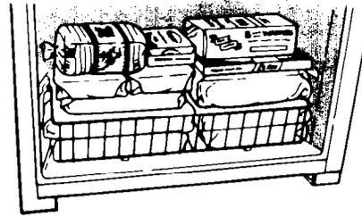
**Baskets** – Store heavy and bulky packages here. Baskets should be in place at all times for proper air circulation.
