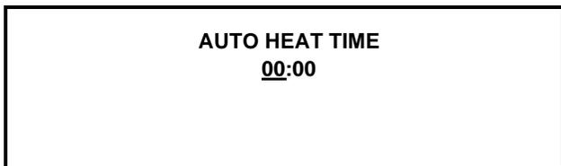
Touch the arrow symbols to increase or decrease the hour to the desired setting. Then move the cursor to the minutes position by touching the SEL symbol. Adjust the setting for minutes. Then touch the SEL symbol to save the setting and return to the AUTO HEAT TIME screen. Touch the SEL symbol to exit the screen and return to the Menu.
