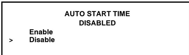
Enable the AUTO START TIME by touching the UP arrow symbol to move the arrow up to Enable. Touch the SEL symbol to advance to the next screen.
