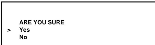
Use the up or down arrow symbol to move the cursor to "YES". Touch the SEL symbol to immediately start a heat cycle.
