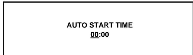
Use the arrow symbols to program the AUTO START TIME by increasing or decreasing the hour setting above the cursor. Touch the SEL symbol to advance the cursor and program the minutes setting. Touch the SEL symbol to return to the previous screen with the new time setting displayed. Touch the SEL symbol to exit the screen and return to the Menu.
