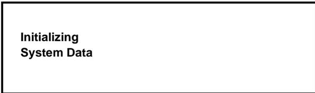
If the System Data is corrupted, the machine is set to OFF, the serving counters are set to zero, and the faults are cleared. A "SYSTEM CRC ERR" fault is set and displayed on the VFD. An acknowledgement (SEL key) is required.
