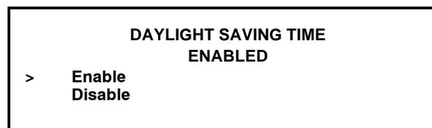
The Daylight Saving feature, when enabled, will automatically adjust the control clock for daylight saving time. To disable the Daylight Saving Time feature, touch the DOWN arrow to move the arrow to "Disable". Then touch the SEL symbol to save the new setting.
