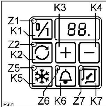
All commands and indicators for the use of the device are grouped in a single control panel placed on the frontal panel. Its functioning is electronically managed in low voltage.
