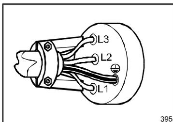
A 4 pole plug, suitable with the current socket, must be installed at the end of the device's power supply cable.
