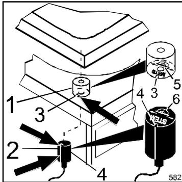
This safety device, featuring an approved type magnet [1] and a magnetic contact [2] avoids accidents caused by the accidental starting of the beater when the lid is open. In consequence the device can't operate when the lid is open, and if it is opened during its functioning the beater immediately stops.
