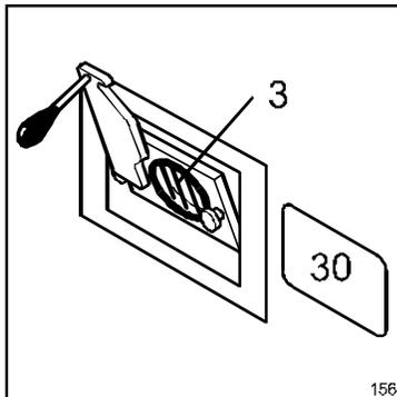
A fixed protection grill [3] prevents, as far as possible, fingers or objects from being **ACCIDENTALLY** inserted in the extraction pipe. In order to insure normal operation it is not possible to adjust the fixed grill as to prevent fingers and objects from being **VOLUNTARILY** inserted through the extraction pipe (**according to Machines Directive 89/392/CEE and ensuing modifications, Appendix I, Art. 1.1.2.b, 3<sup>rd</sup> paragraph**).
