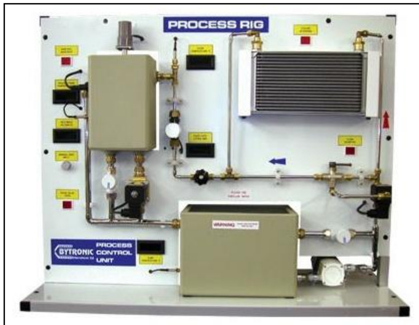
Figura 1 – Painel real do Process Rig [1]
