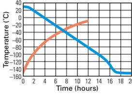
Ambient temp. and maintenance of -135°C by injection of LN<sub>2</sub> (50kg)
