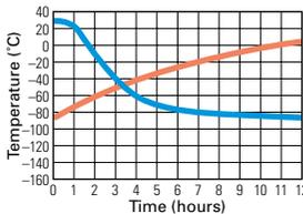
Ambient temp. and maintenance of -70°C by injection of LCO<sub>2</sub> (30kg)
