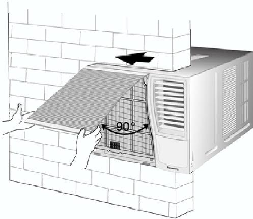
**Caution:** Do not raise the front intake grille any higher than 90° to the unit or damage to the tabs may occur.
