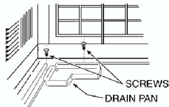
Install the drain pan at the left corner of the cabinet using 2 screws.
