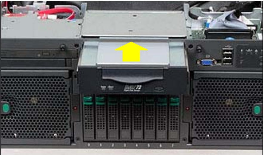
Figure 22: Inserting the tape drive
