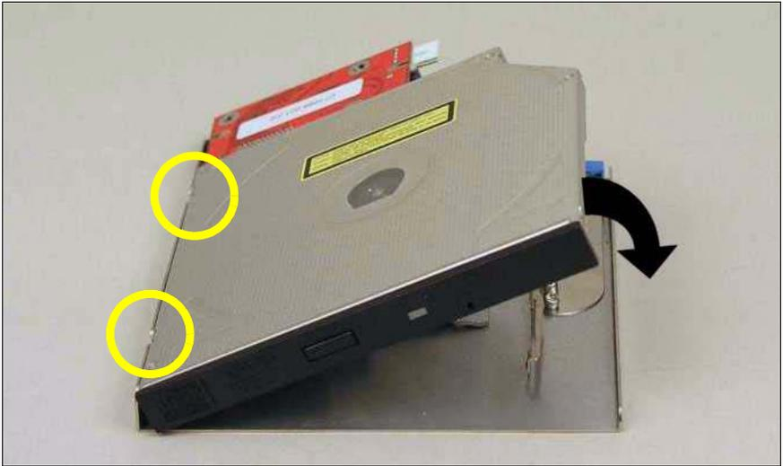
Figure 16: Mounting the drive in its frame
