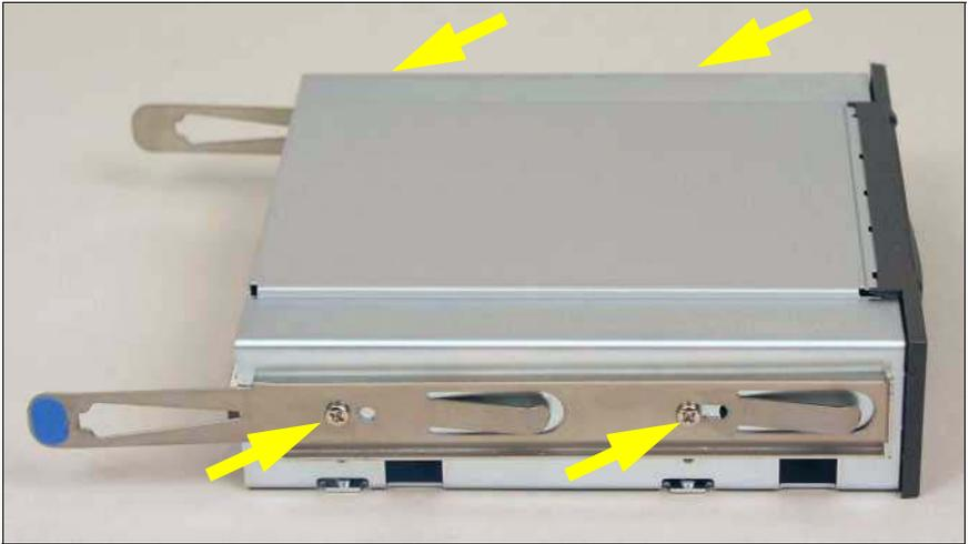
Figure 21: Fastening the sliding rails on the drive
