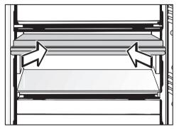
■ Take out the third drawer down and push the isolation plate in **under** the second drawer.
