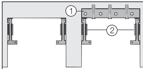
If the installation niche is deeper than the appliance, a solid wooden beam (1) can be placed behind the anti-tip brackets (2) so the appliance can be securely attached to the base or wall.
