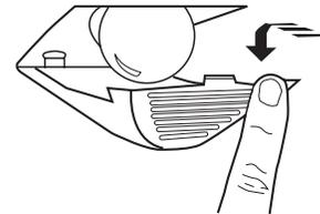
3. Replace the light bulb with an appliance bulb of the same wattage.
