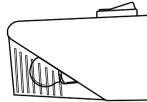
2. Replace the light bulb with an appliance bulb of the same wattage.
