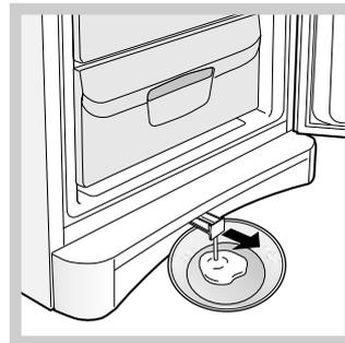
5. Certain appliances are fitted with the DRAIN SYSTEM to lead the water outside. Let the water flow into a container (see diagram).
