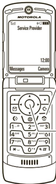
① Press and hold the **Power Key**
