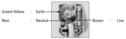
If you change the plug, the colour of wires in the mains lead may not correspond with the colour of the markings identifying terminals in the plug. You should therefore wire it as shown above.
