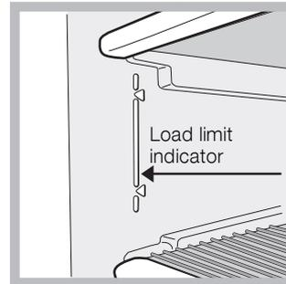
If the top drawer is not used DO NOT store food beyond the line embossed in the interior of the freezer cabinet wall. This indicates the load limit. Food beyond this line will limit the air circulation and affect the performance of the freezer.
