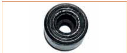
interior ring damaged for 100%
