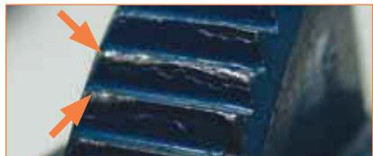
1 tooth damaged for 100% and 1 teeth damaged for 50%
