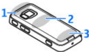
1 — Antena Bluetooth e LAN sem fios (WLAN), e receptor GPS
