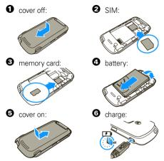
Note: You may need to charge your phone overnight before using it for the first time. If the battery is completely drained, the display will not turn on, but you will see a small red light by the camera lens.
