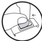
◆ Remove the protective film from the bracket and affix it in the chosen area.
