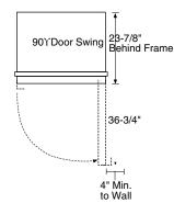
Allow 25" minimum clearance for a full 130° door swing. Allow 15" for pan removal. for a 90° door swing, allow 4" minimum clearance for professional models. If the 90° doorstop position is used, pan access is maintained but pan removal is restricted.
