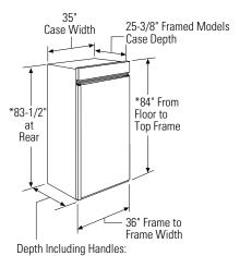
\*Shipping height. The freezer can be adjusted to fit into a cutout 83-1/2" min. to 84-1/2" max. height. Note: the top case trim at the front is 1/2" higher and will overlap upper cabinetry or soffit. Use leveling legs and wheels for a maximum 1" height adjustment.
