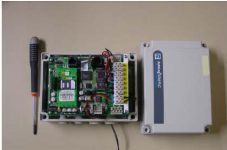
Pic.4 AutoLog GSM4 Unit with IP65 enclosure
