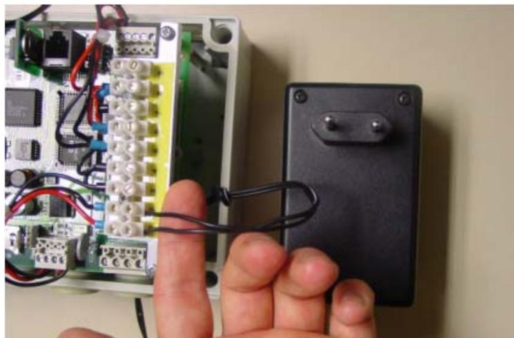
Check that power supply (12-24 VDC) has been connected to GSM-PLC
