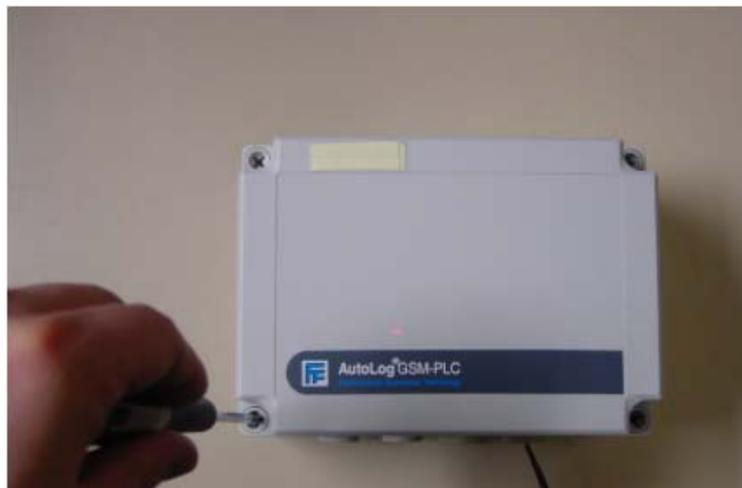
Pic.2 Open the cover with screwdriver (GSM4 Unit on picture)
