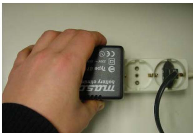
Connect power supply to electrical network
