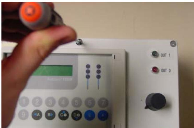
Pic.3 Open the cover with screwdriver (GSM14 Unit in picture)
