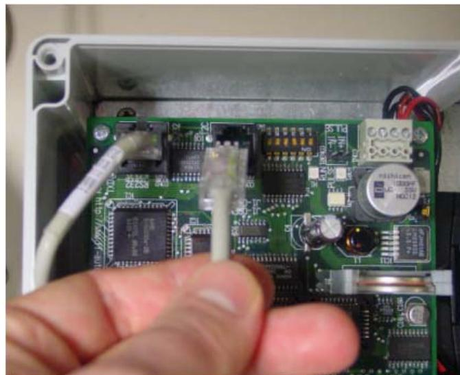
If you have the control panel, connect it to I2C connector (GSM14 Unit in picture):
