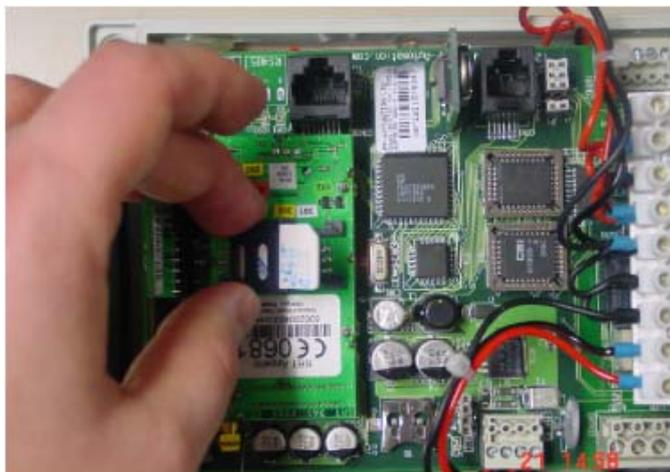
Connect power on and check RX, TX, RUN and SERV leds, they should blink.
