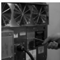
5. Using a Phillips screwdriver, remove the screws from the rear vent catalyst housing. Support the cover with your hand.
