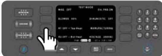
Figure 21: Test Mode: Top Heater Test
