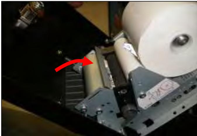
Pull the paper through the slot on the door and close the small metal guide.
