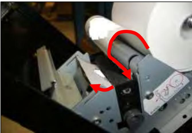
Run the paper under the rubber roller and back out the other side.
