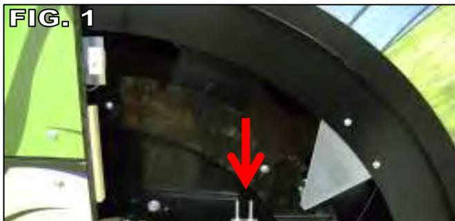
3. PULL EACH BOLT UP AND SPIN THE LOCK-NUT TO ADJUST. YOU ONLY NEED TO DO 2 REVOLUTIONS TO ALTER THE PRESSURE.
