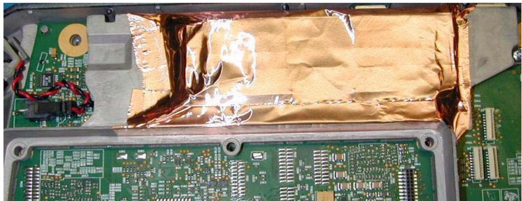
**Figure 4.16 Copper Tape Installation**
