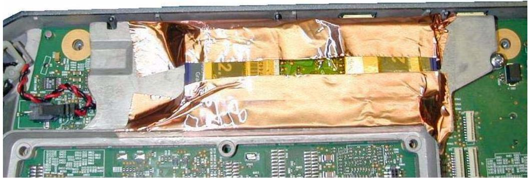
**Figure 4.15 Copper Tape Installation**
