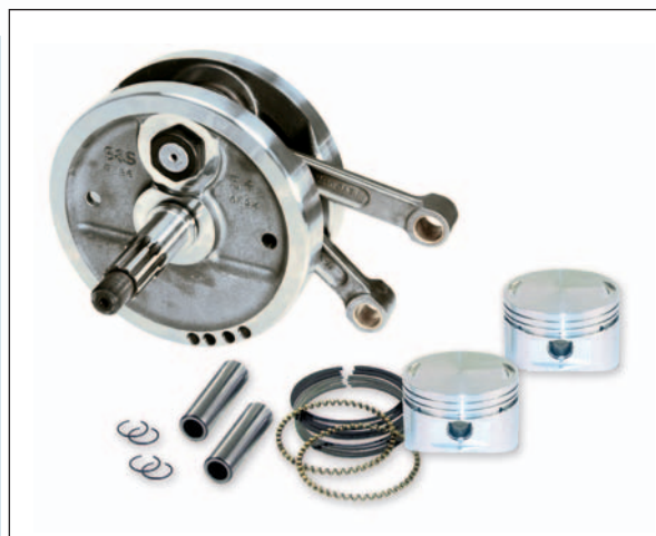
Big Twin stock bore stroker kit shown here complete and assembled. 32-2489
