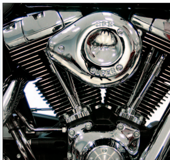
S&S Teardrop Induction System features the classic S&S Teardrop high flow air cleaner.
