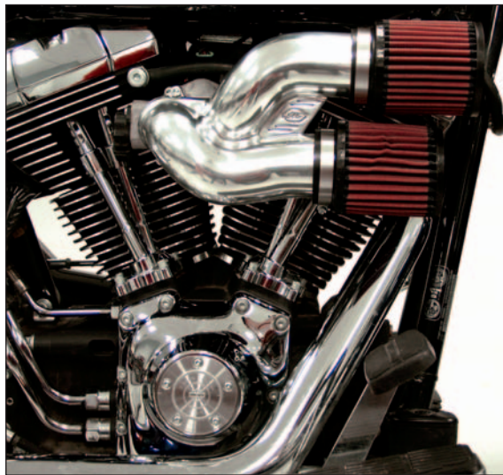
S&S VFI Tuned Induction System features dual independent tuned intake tracts, one for each cylinder.
