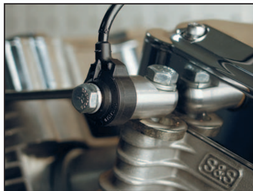
Exclusive S&S knock sensor installed on cylinder head top motor mount. No other ignition system for V-Twin motorcycles uses knock sensing to control ignition timing.
