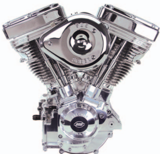
Polished SSW+ Engine with S&S IST Ignition system. IST equipped engines carry an extra year of warranty. Note the special billet gearcover.
