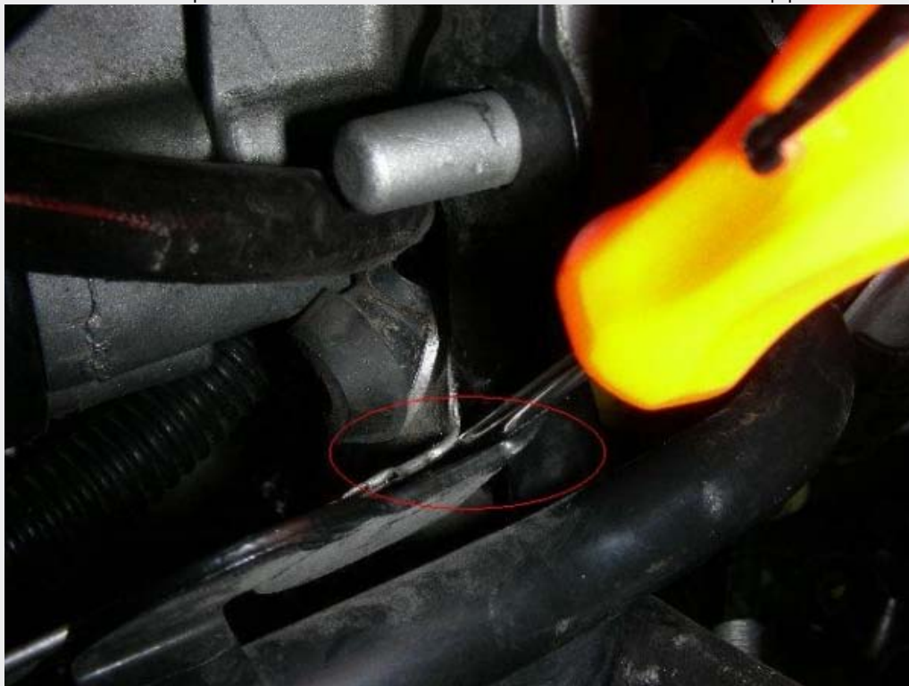
Either during manufacture or when the engine harness was replaced locally, the installer had become impatient with the heat shield and forced it in place, bending the shield, missing the grommet mounts, and abrading a starter wire & powersteering cables.
