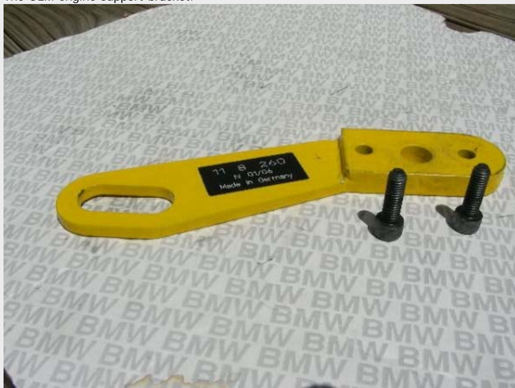
Some filing of the bracket is needed in order for it to fit behind a coolant hose.
