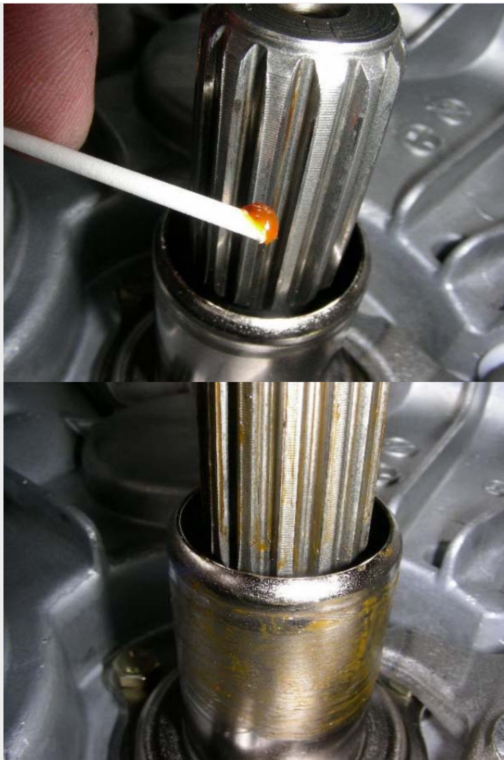
A final inspection to make sure the clutch release bearing is in its place before bolting up the gear box.
