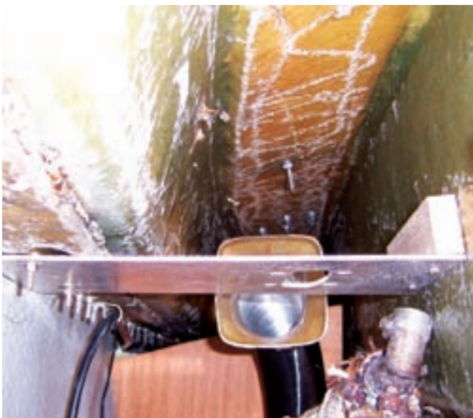
Tony found the ideal location for the heater in the unused space under the port-side cockpit coaming, at left, and made an aluminum shelf to support it. He also had to make an adaptor to connect his consignment-store heater to the air ducting normally used in boats, at right.
