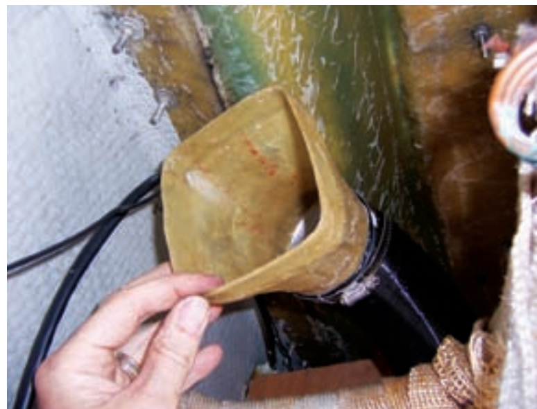
Tony found the ideal location for the heater in the unused space under the port-side cockpit coaming, at left, and made an aluminum shelf to support it. He also had to make an adaptor to connect his consignment-store heater to the air ducting normally used in boats, at right.
