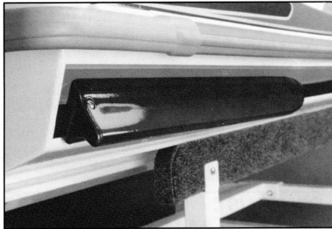
exit nozzle does not need mounting bosses for the nozzle trim pivot points. Because of this, the exit nozzle from the JS750SX is used. A quick-turn steering nozzle incorporating a vertical vane for more responsive cornering completes the XiR pump. The XiR generates
