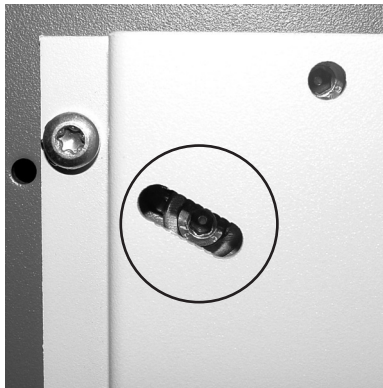
Bottom of cell washer with imbalance adjustment screw circled
