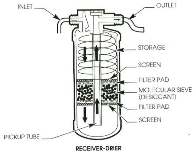
*Inside the receiver/drier, desiccant absorbs any excess moisture from the refrigerant.*
