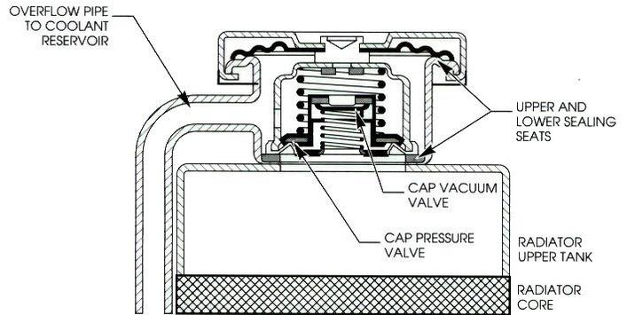
The pressure radiator cap seals the cooling system at the inlet on top of the radiator. Caps are pressure rated to match cooling system design. Each pound of pressure on the cooling system raises the boiling point of coolant three degrees Fahrenheit, so the pressure cap extends the cooling system operating range above the normal boiling point. The cap pressure valve opens when operating pressures are high. Coolant can flow through the heater core regardless of thermostat position.
