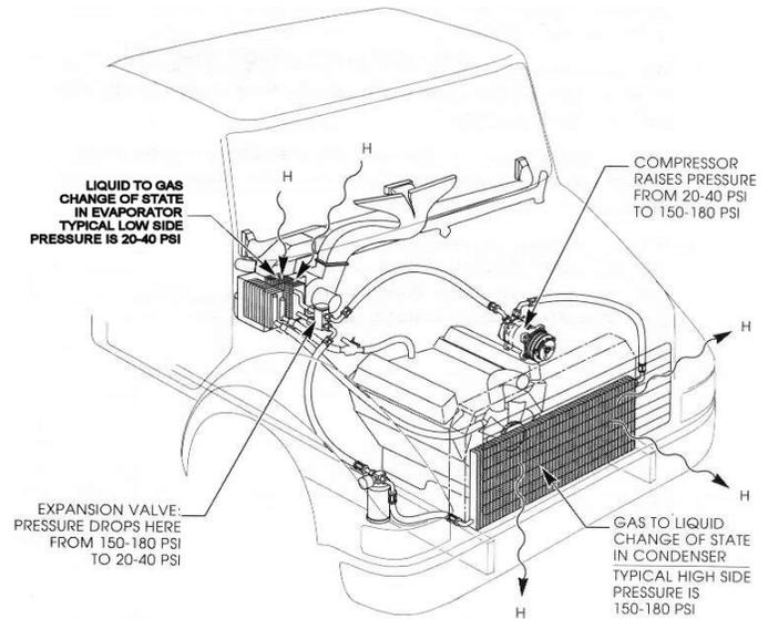
*Warm air moving past the evaporator provides the heat necessary for the low-pressure refrigerant to boil and change states.*
