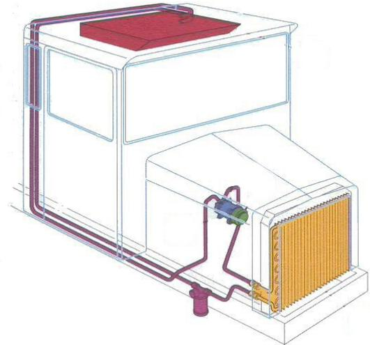
*The hot, compressed refrigerant leaves the compressor and enters the condenser. Air blowing past the condenser coils carries away the excess heat, allowing the refrigerant to condense back to a liquid.*
