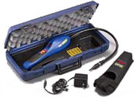
*Electronic leak detectors enable you to find leaks as small as a couple of ounces of refrigerant per year. Early R12 detectors can't detect R134a...make sure you're using the right type of leak detector for the system you're working on.*
