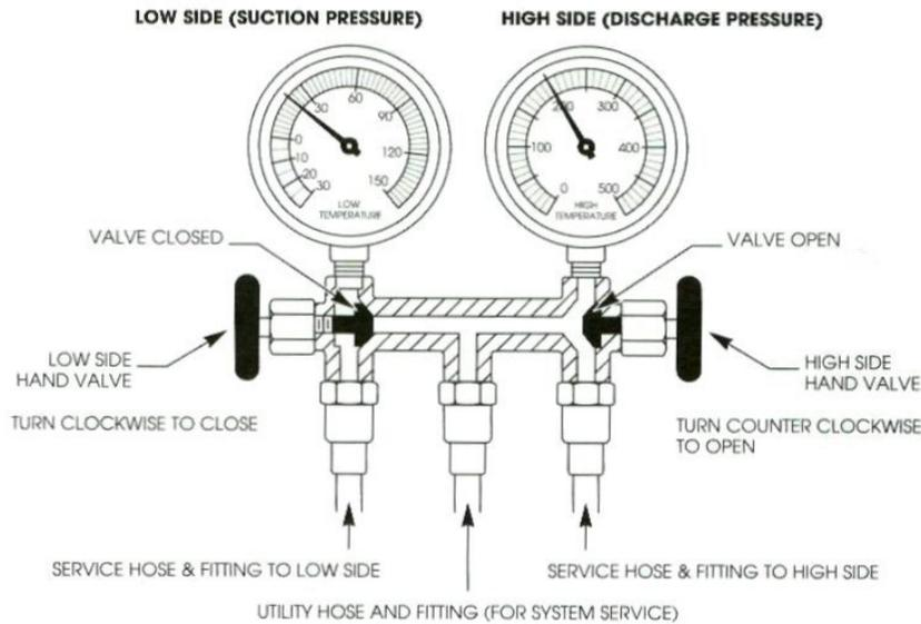
*The low pressure gauge displays pounds per square inch (PSI) and inches of mercury (in. Hg). Hg is the chemical symbol for mercury. The high pressure gauge reads in pounds per square inch.*
