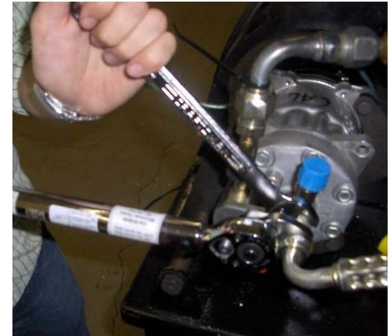
Tighten connection with proper torque.
