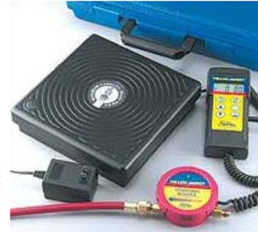
*Because of the possible mixing of different refrigerants, it's important that you have a dedicated set of service equipment for each system. This prevents the possibility of system contamination.*
