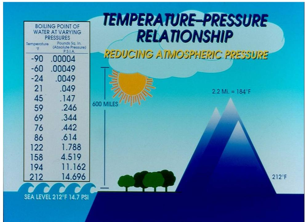
Water doesn't necessarily boil at 212°F, or 100° C - pressure affects boiling temperature. By increasing system pressure, boiling temperature increases.
