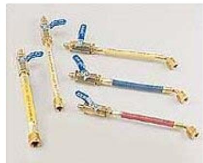
*Whether you're using gauges or a recycling machine to service or diagnose a system, you must have shutoff valves no more than 12" from the ends of the hoses.*
