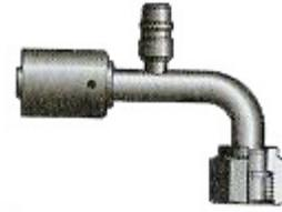
*All the caps for the service ports screw on, and each cap has an O-ring inside. These caps are the primary seal for service ports.*
