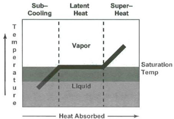
*Latent heat is the heat required to make a liquid at a certain pressure turn into a vapor at that pressure. The saturation temperature changes with the pressure of the refrigerant.*
