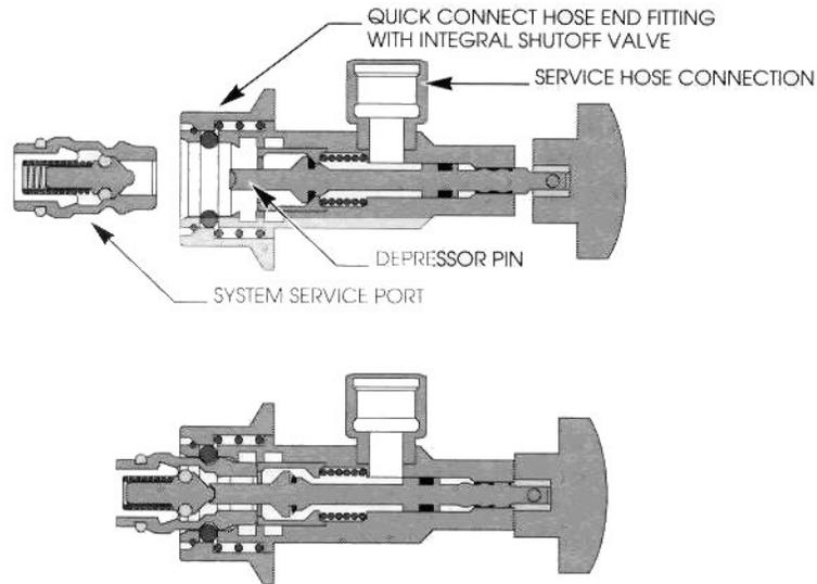
VALVE ASSEMBLED TO SERVICE PORT WITH VALVE IN THE OPEN POSITION
