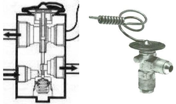
*The expansion valve restricts the flow of refrigerant, to provide the pressure differential the system needs for the refrigerant's temperature and boiling point to increase and decrease.*
