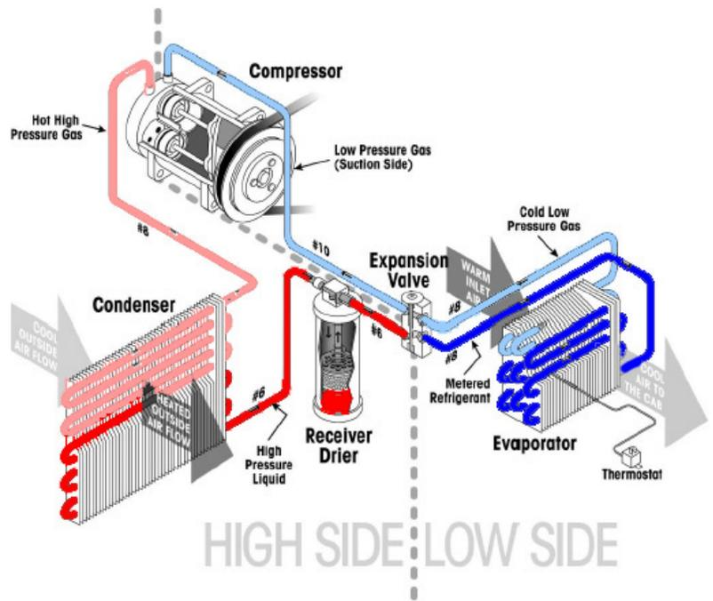
*The air conditioning system is divided into two sides, the high side and the low side. This illustrates the flow of refrigerant through the system.*
