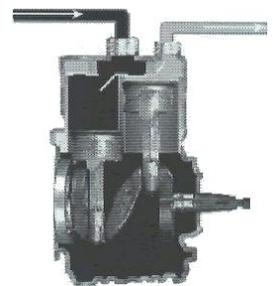
*The compressor pumps the refrigerant through the system to provide flow.*
