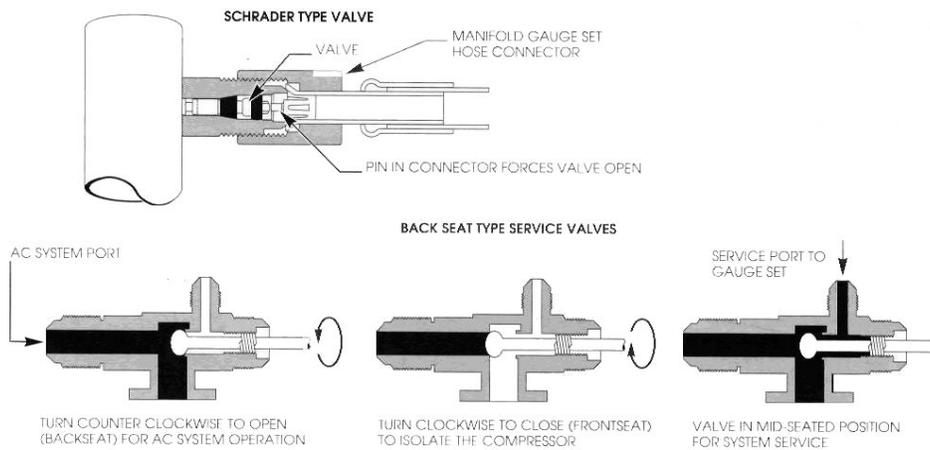
*The valve drawings are cutaway. The Schrader valve in the upper portion of the illustration (like a tire air valve) is either closed or open. The three illustrations above show and describe stem type valve operations.*
