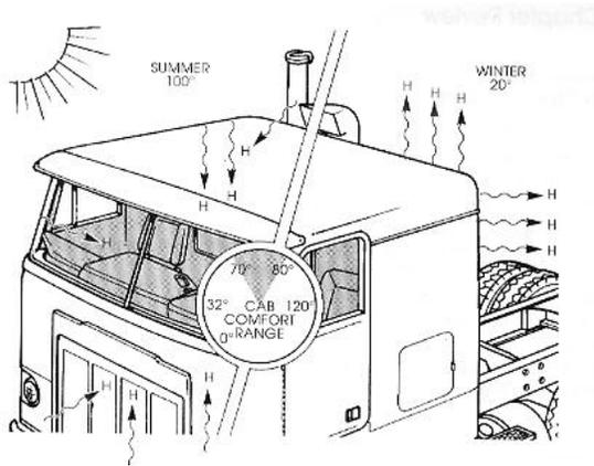
*This drawing shows how heat moves; one of nature's laws. Heat always moves from a warm to a cool area – heat flows into the cab in hot weather and flows out in cold weather.*
