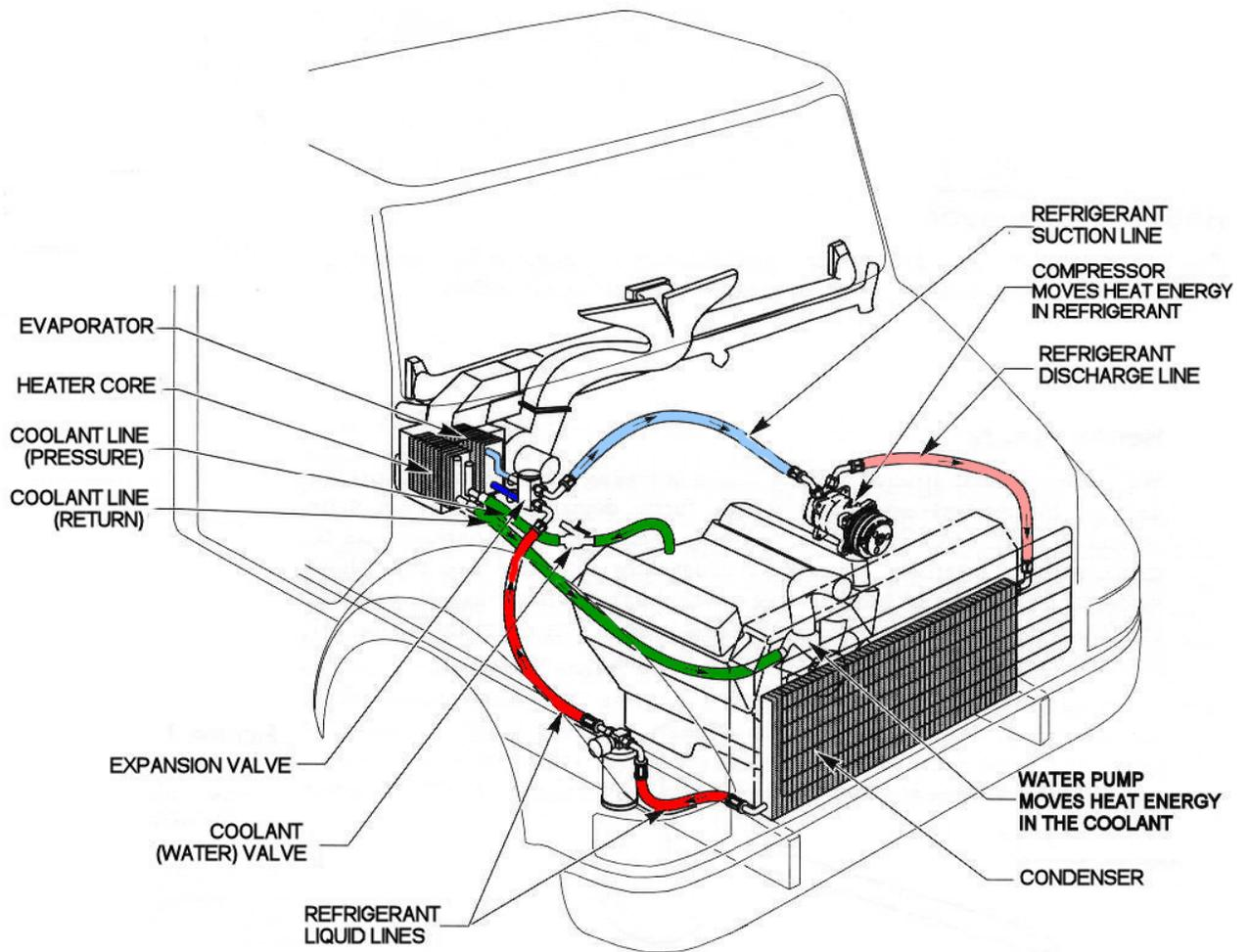
This picture shows the direction of refrigerant and engine coolant flow in the system. The air conditioner evaporator coil and condenser, and the heater core, are the main points of heat transfer.
