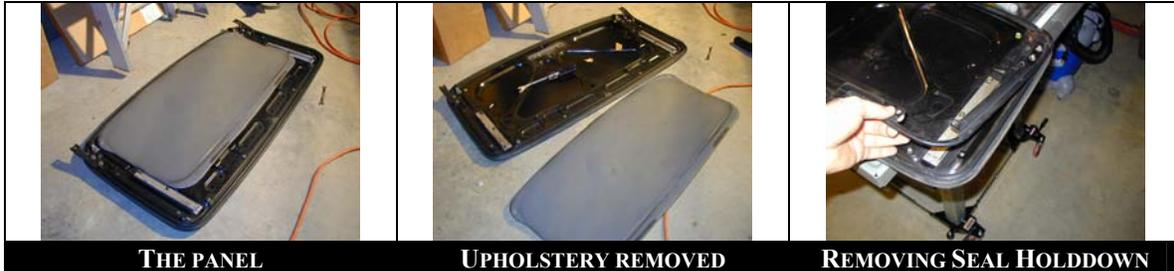
With the sunroof panel on the workbench, flip it over so that the upholstery is exposed. Remove the 2 philips head screws and then CAREFULLY pry the upholstery panel from the metal panel. There is one plastic rivet in the middle of the upholstered panel that is hard to break loose without tearing the panel. Mine tore out so I will just put it back without it.
