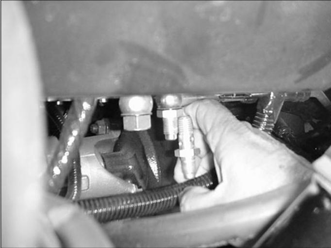
On the inside, the part with the rifled opening attaches the fuel line to the fuel pump. On the outside, the Schrader valve (think A/C valve or, better yet, a tire valve) has a press-for-pressure needle. Here is the catch, you can take the pressure needle out of the Schrader valve.
