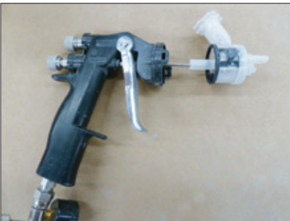
Top —The PPS units attach directly to most spray guns or through adapters available from 3M. Above —The Accuspray model HGO9 from 3M offers additional disposability in its hard plastic atomizing spray nozzle, which removes easily and can be reused, or replaced for $20.
