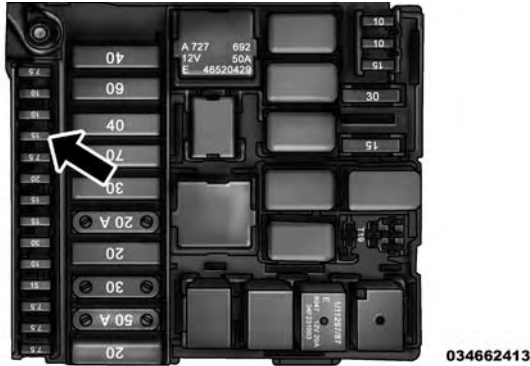
Power Outlet Fuse Location Underhood
