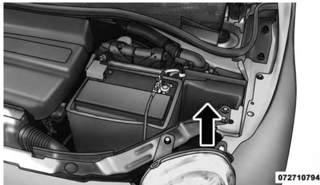
Front Distribution Unit
