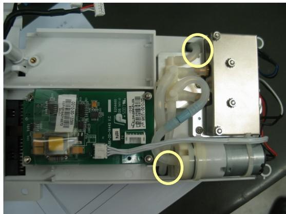
3. Unscrew the three M3×6 screws and pull up the multi-parameter board.
