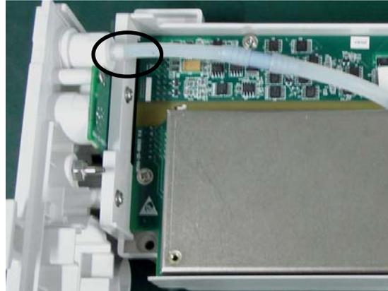
2. Unscrew the three M3×6 screws to take out the front panel assembly.
