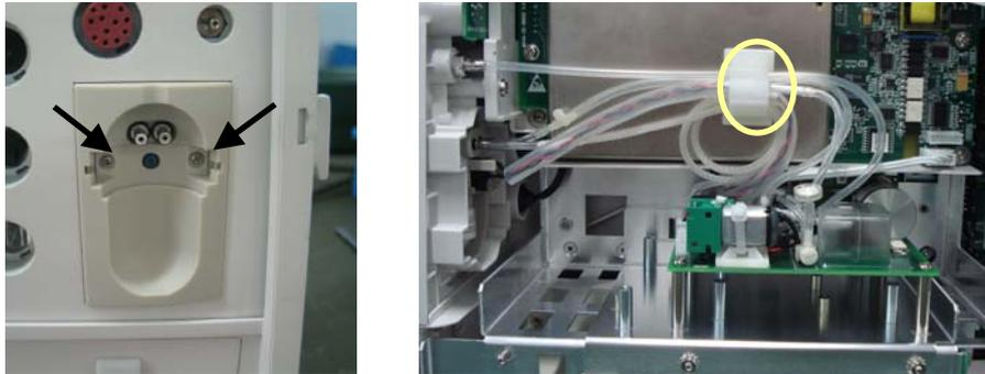
2. Take out the watertrap assembly and move it through the fixer in the way as shown below.
