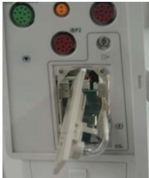
3. Unplug the communication cable from the multi-parameter board. Unplug the tubing from the gas nipple. Then unscrew the two nuts and pull out the Mindray CO2 assembly.
