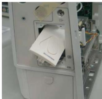
3. Unplug the communication cable from the multi-parameter board. Unplug the tubing from the gas nipple. Then unscrew the two nuts and pull out the microstream CO2 assembly.
