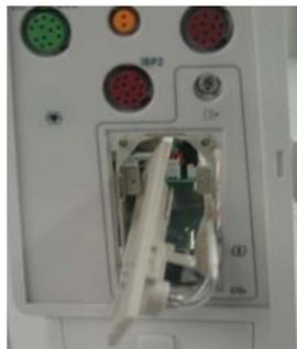
3. Unplug the cable from the multi-parameter board. Unplug the tubing from the gas nipple. Then unscrew the three nuts and one screw and pull out the AG assembly.
