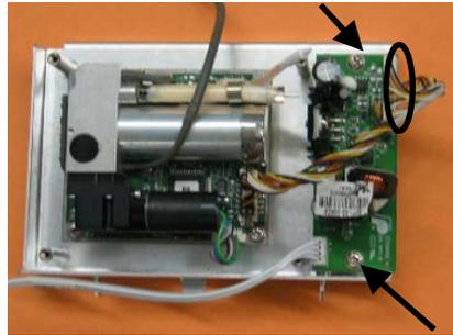
Unscrew the four M3×6 screws to take out the microstream CO2 module.
