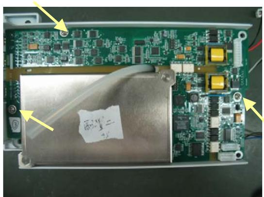
4. Unscrew the two M3×6 screws to take out the ECG shield.
