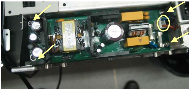
3. Cut the three 3×80mm cable ties and unscrew the two M3×6 screws to take out the fan assembly. Unscrew the two M3×6 screws to take out the speaker assembly.
