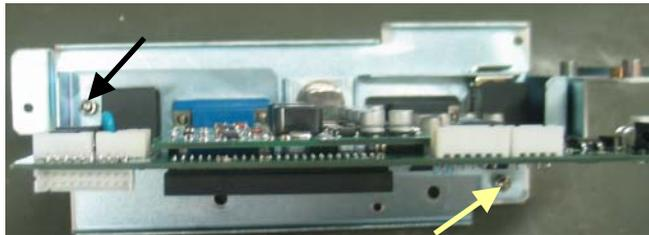
2. Take out the beryllium copper leaf and unscrew the four stud screws and one BNC nut to take out the interface board inner support rack.
