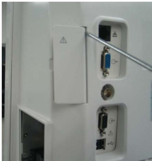
2. Open the battery door. Then poke the pin out with a flat-bladed screwdriver.
