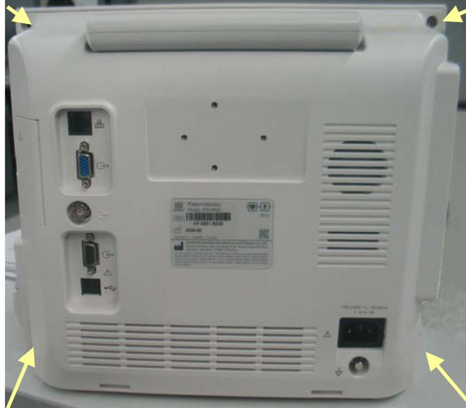
2. Pull out the front housing gently. Disconnect the cable connecting the power management and interface board and the main board. Then the front and rear housing can be separated.
