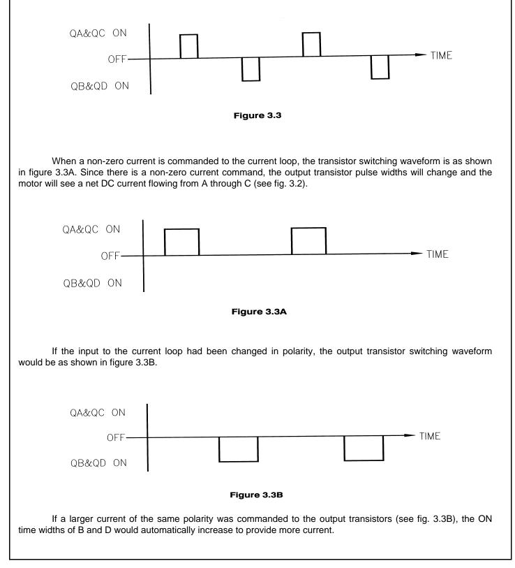
From the previous examples it is easy to understand why this output transistor switching technique is referred to as Pulse-Width-Modulation.
