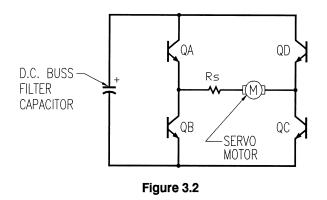
The advantage of an AH TYPE<sup>®</sup> output bridge configuration is that by controlling the switching of the opposite pairs of transistors, current can be made to flow through the motor in either direction using a single polarity power supply as shown in figure 3.2.
