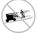
Limit travel speed according to condition of ground surface, congestion, slope, location of personnel, and any other factors which may cause collision.
