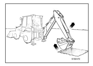
Swing the bucket towards the dump area. Start dumping as the bucket approaches the pile. Do not waste time by dumping too far from the excavation. Dump close to the start dig position. Swing the bucket back to the excavation and start the next dig.
