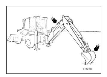
When the bucket is full, close it fully and at the same time move the dipper out a little way. This will keep soil from building up under the machine.
