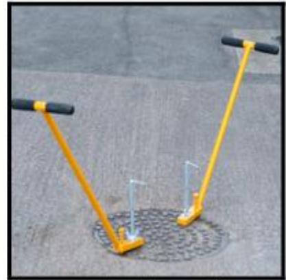
(2-man manual manhole cover lifting arms)
