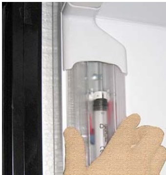
Remove Shield from Display Lamp
