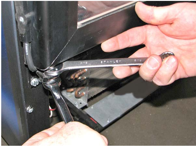
Adjust Door Closing Torque
