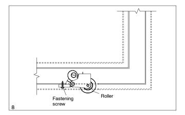
NOTE: These rollers are marked right and left and must be installed as viewed from interior. Rollers have an identification stamped on them. See illustration 9.
